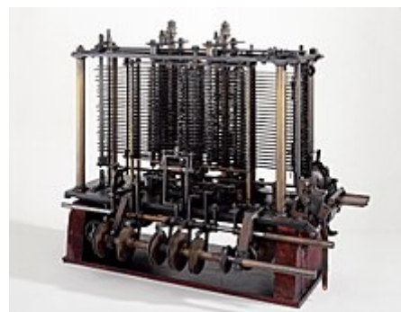
Portion of the mill with a printing mechanism of the Analytical Engine, built by Charles Babbage, as displayed at the Science Museum (London)
